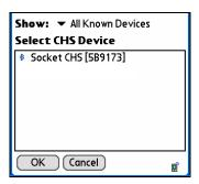
The Cordless Hand Scanner will appear as Socket CHS [xxxxxx], where the characters in brackets are the last 6 characters of the scanner's *Bluetooth* MAC address. If multiple Cordless Hand Scanners were detected, identify yours by checking the MAC address printed on a label in the battery compartment.
